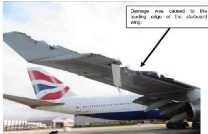
Figure 4 Damage caused to the starboard wing of the BA034 aircraft
