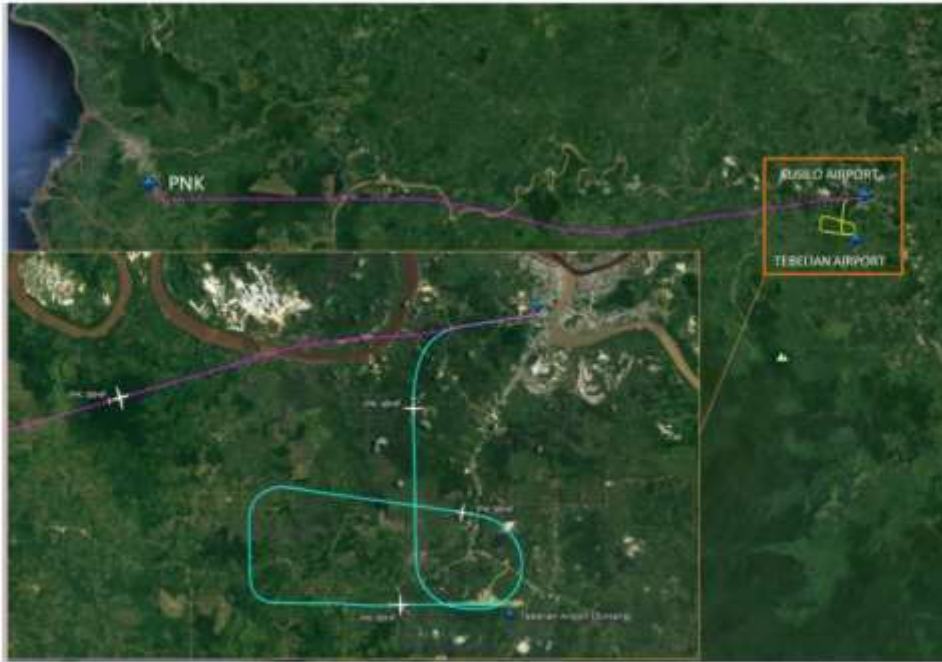
Figure 2: The flight track as recorded on the FDR. Purple line indicated the flight from Pontianak to Susilo Airport, and the blue line indicated the flight from Susilo Airport to Tebelian Airport.
