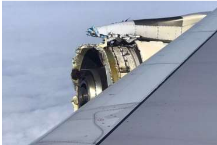
uncontained engine failure
