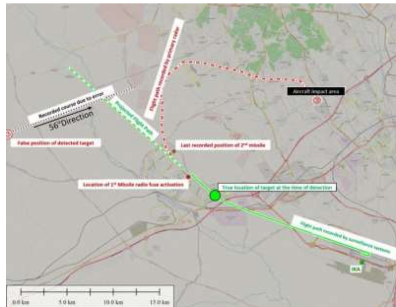
Complete flight trajectory and missile last positions (Graphics: Iran's AIB)
